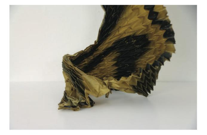
The creation of the pleated sensor involves five steps. First - folding two identical origami molds out of paper.
