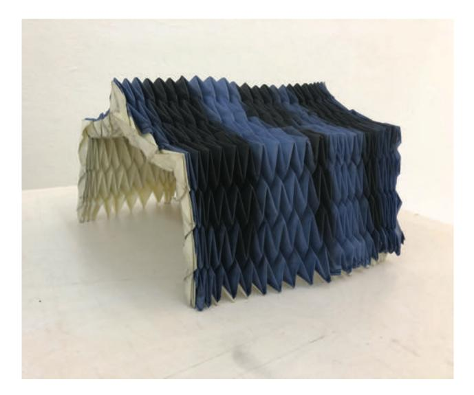
Let the closed mold cool down completely. For the bigger samples and the final prototype some kind of reinforcement was needed to keep the folds as stiff and clean as possible. Here, a clear spray lacquer was applied after opening and removing one side of the mold.
