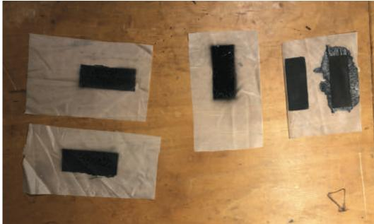
After cutting the fabric, the graphite spray paint is applied either using stencils for a structured/geometric result, or freehand for a more organic one.
