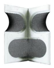
Based on previous work on hinge constructions made from 3D prints on textiles, the intention here is to use the tensile hinge as a basic construction that is suitable as a sensor for sound installations and conveys a more organic aesthetic.
