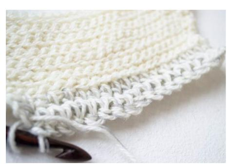
Crochet detail (White wool and Light grey Bekinox Conductive yarn BK50/2 Nm50/2 80% Polyester 20% stainless steel.
