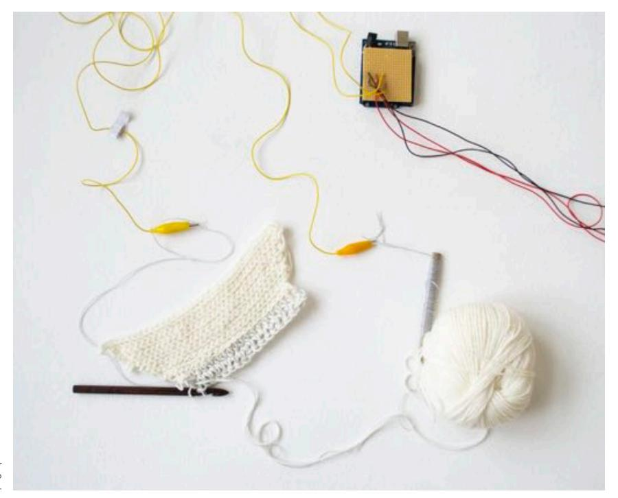
Crochet Sensor connected to Arduino.
