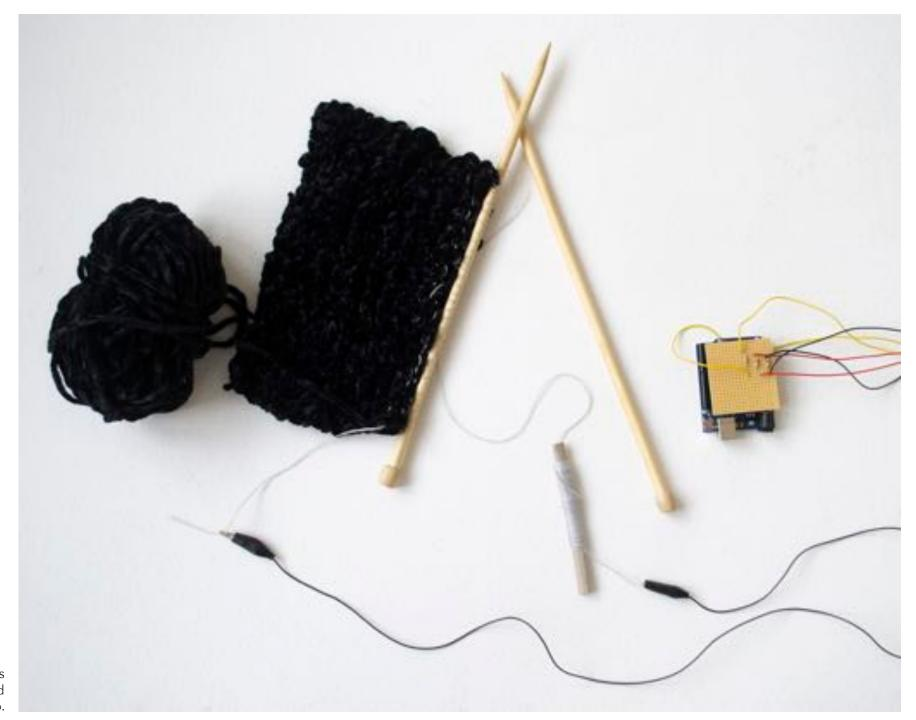
Knitting Needles sensor connected to Arduino.
